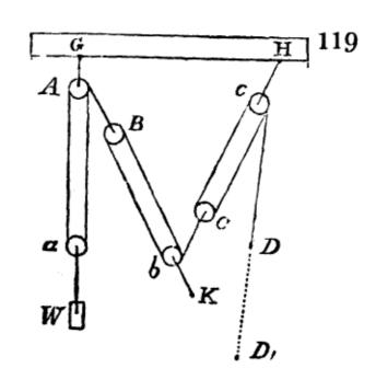
block of a tackle in which there are  $n_1$  strings at a, and of which AB is the fall; let the extremity of this fall be tied to the moveable block B of a second tackle of which b is the fixed block, and  $n_2$  the number of strings at B. Also, let the fall bc of the second tackle be tied to the moveable block C of a third tackle of which c is the fixed block, and cD the fall, and  $n_3$  the strings at C; let a velocity  $V_4$  be given to
